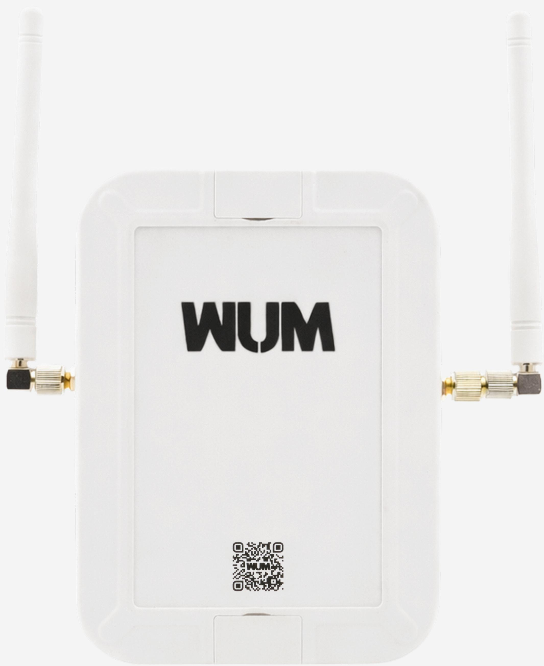
The device simultaneously operates as a full-featured LoRaWAN concentrator and as the root node in proprietary LoRa Mesh networks, at both hardware and software levels. It enables hybrid network deployments with extended radio coverage, high scalability, and robust fault tolerance in demanding RF environments.
