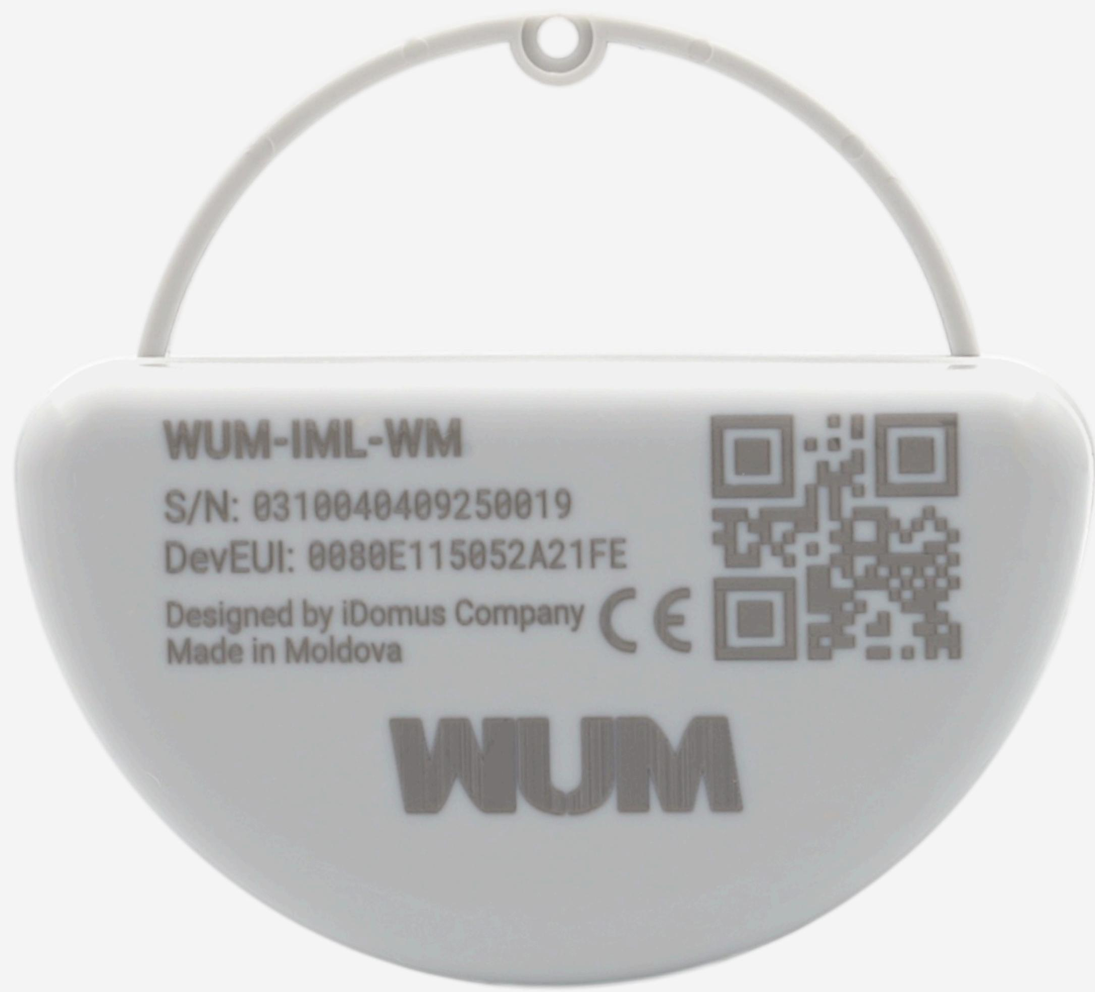
The **WUM**-IML-WM Pulser module is powered by a long-life battery.
