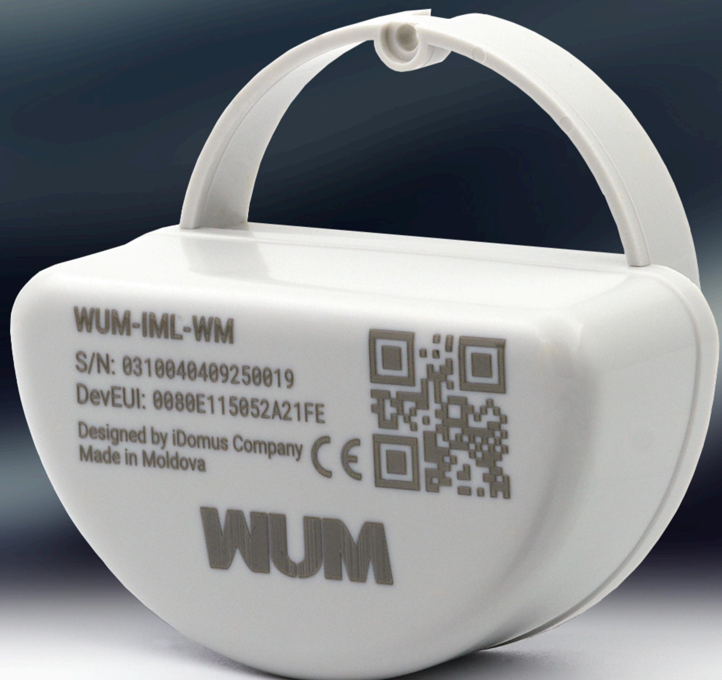
**WUM-IML-WM Pulser** is a wireless IIoT device with internal configurable logic, designed for remote monitoring and data acquisition from water meters (manufactured by Madalena& Servostal) by pulse reading with a Hall sensor and wireless data transmission via LoRaWAN network.
