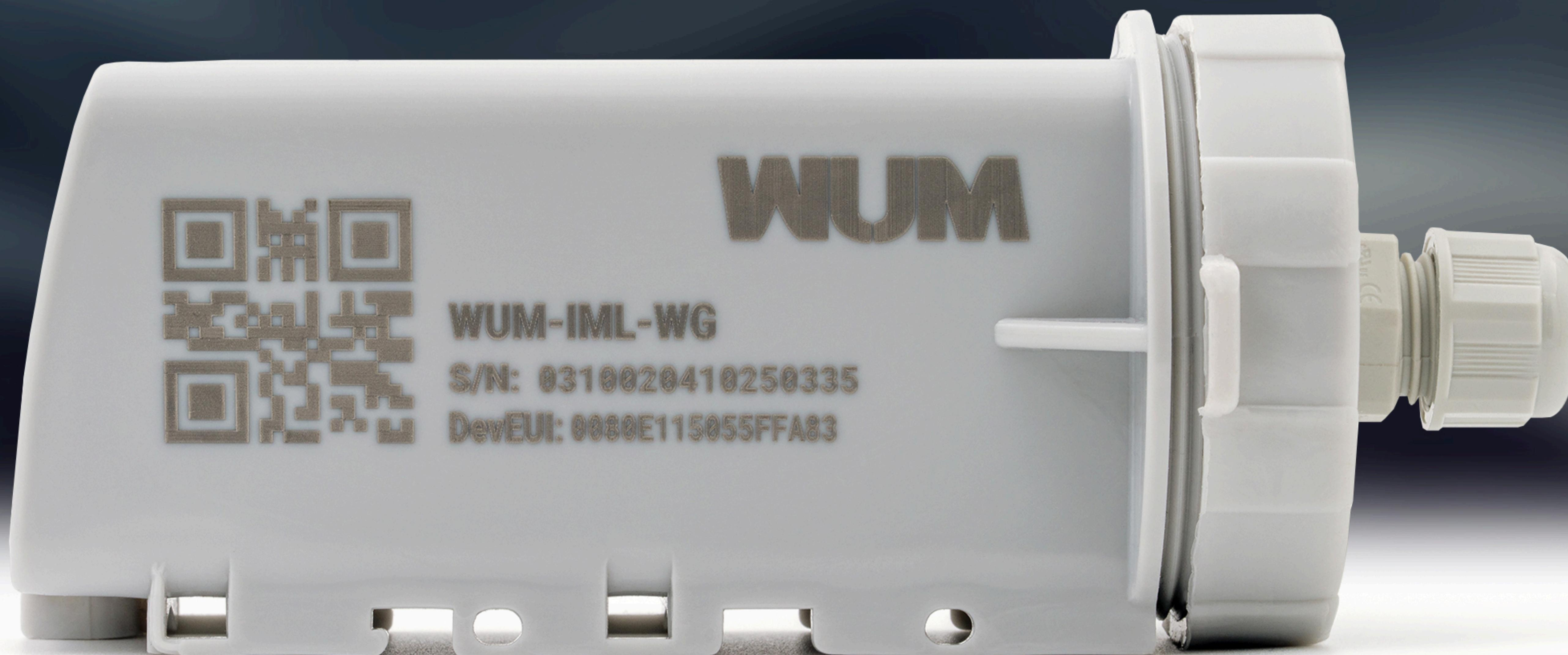
**WUM-IML-WG Pulser** is a wireless IIoT device with internal configurable logic, designed for remote monitoring and data acquisition from water and gas meters via pulse output, with wireless transmission over the LoRaWAN network.
