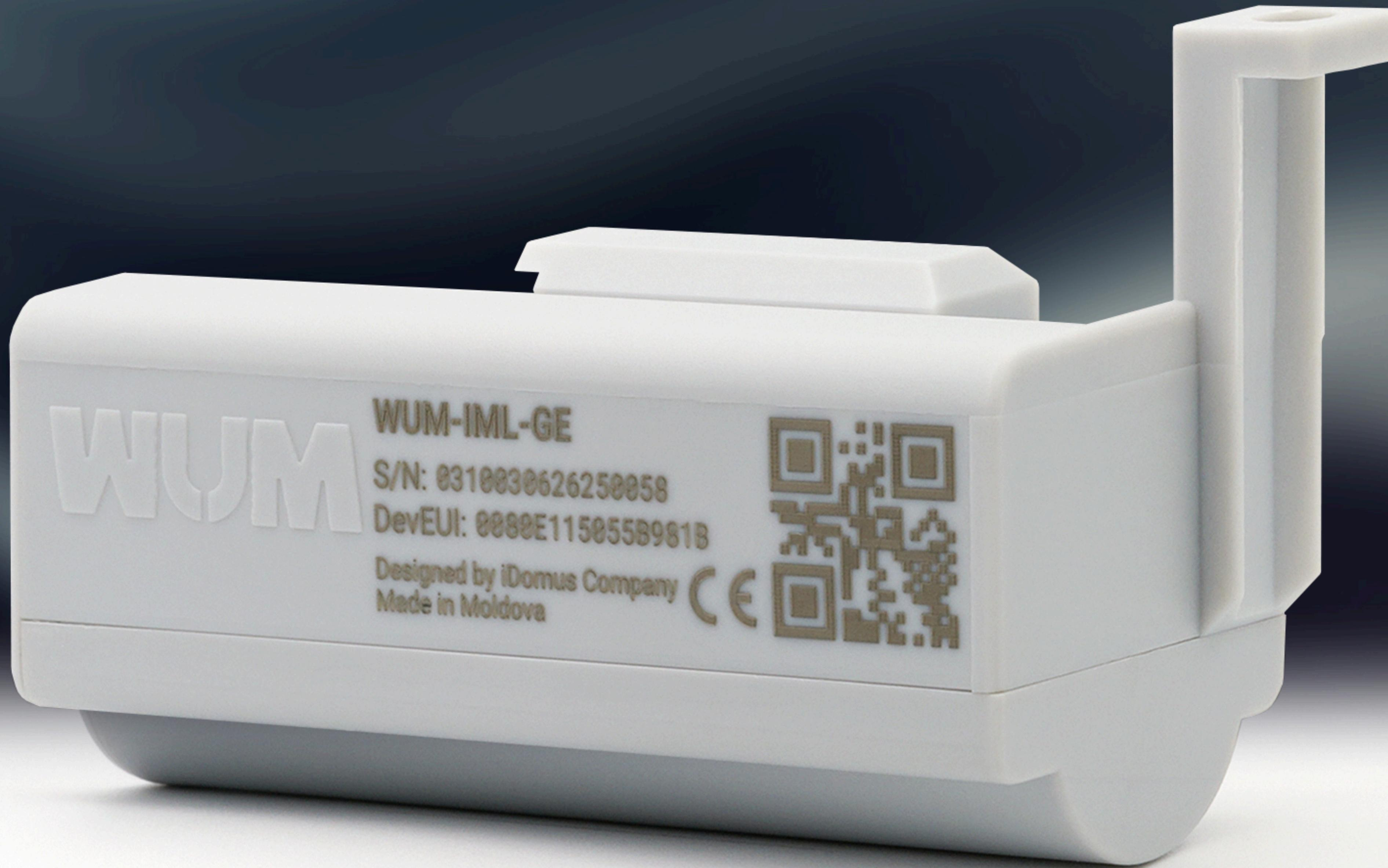
**WUM-IML-GE Pulser** is a wireless IIoT device with internal configurable logic, designed for remote monitoring and data acquisition from Elster, Honeywell, and PremaGas gas meters via the pulse output, with wireless transmission over the LoRaWAN network.
