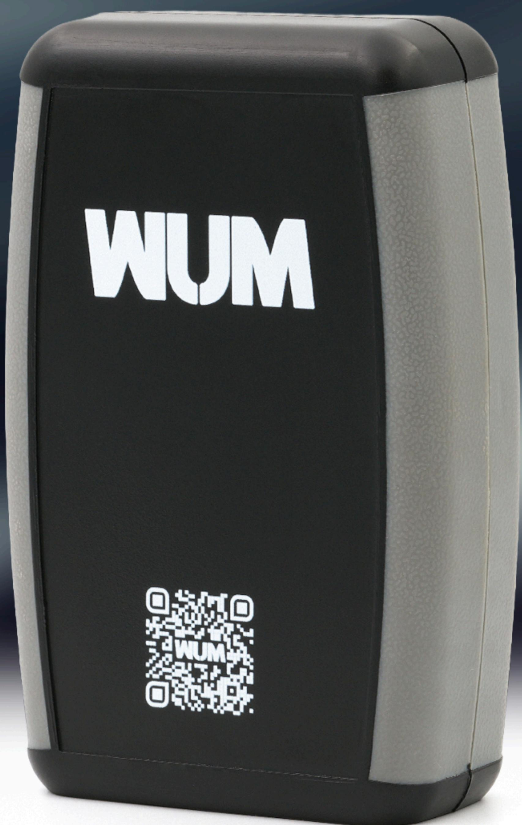
**WUM**-CFG is a portable device specifically designed for remote configuration, control, and setting of the entire range of IIoT devices developed and produced by iDomus, via a dedicated mobile application.
