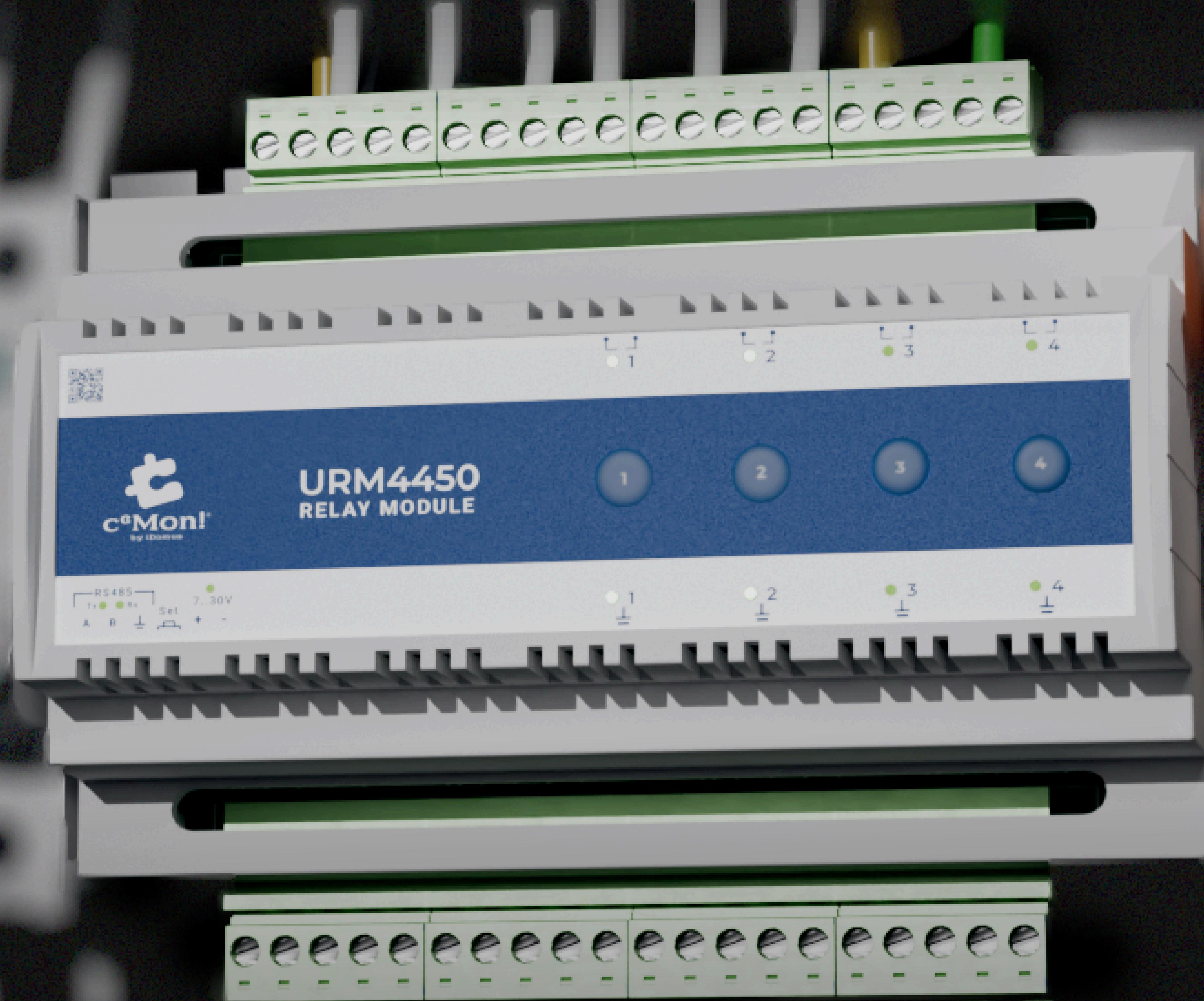
CMN-URM-4450 is a universal industrial relay module featuring an RS-485 interface and support for the Modbus RTU protocol. The module is designed for automated control and monitoring of **energetic infrastructure components**, distributed street lighting systems, BMS, and energy resource dispatch systems.
