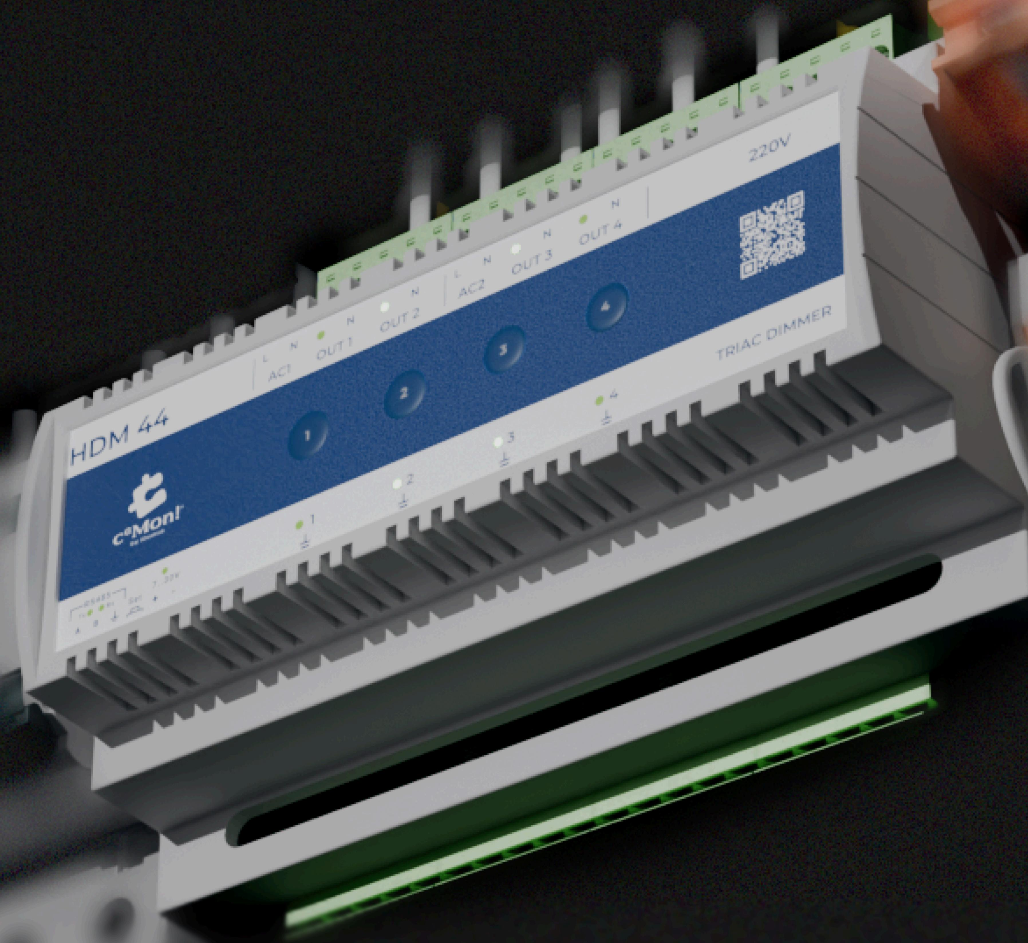
CMN-HDM-44 is an industrial high-voltage TRIAC dimmer, handling 220 V AC loads and featuring RS-485 interface and Modbus RTU protocol support. The device is designed for stepless dimming and on/off control of lighting loads in automation systems, BMS, smart home installations and industrial lighting control systems.
